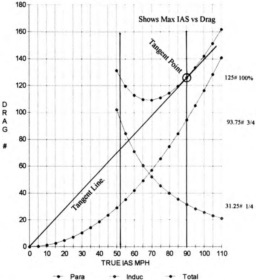
Now if Drag, Fuel Used, and \$ Cost are all equivalent, you can see that tangent point is MAX SPEED PER \$ --- except that we're going to go much faster by climbing high, (TAS), then we're going to maximize engine efficiency, minimize fuel burn, spend much less on fuel, high, by getting the engine wide open and leaned. SPEED / \$ IS MAX HIGH! ✓
