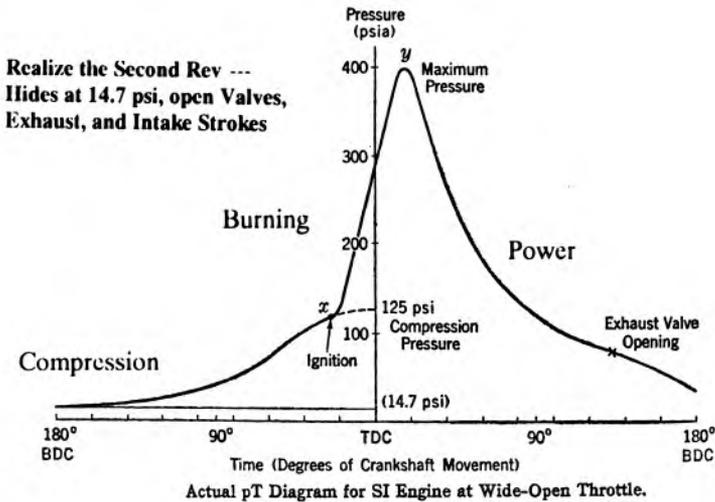
The PV, Pressure, Volume, and the PT, Pressure, Time Diagrams for a Spark Ignition Engine. A **Four Stroke Engine** takes **Two Revolutions** -- **Intake, Compression, Power, Exhaust**. This page emphasizes the Actual **Compression**, (burning), **Power** Revolution, the **Exhaust, Intake** on the Second Revolution, nominally at the 14.7 psi Atmospheric Pressure line. The next Throttled drawings makes it more clear.
