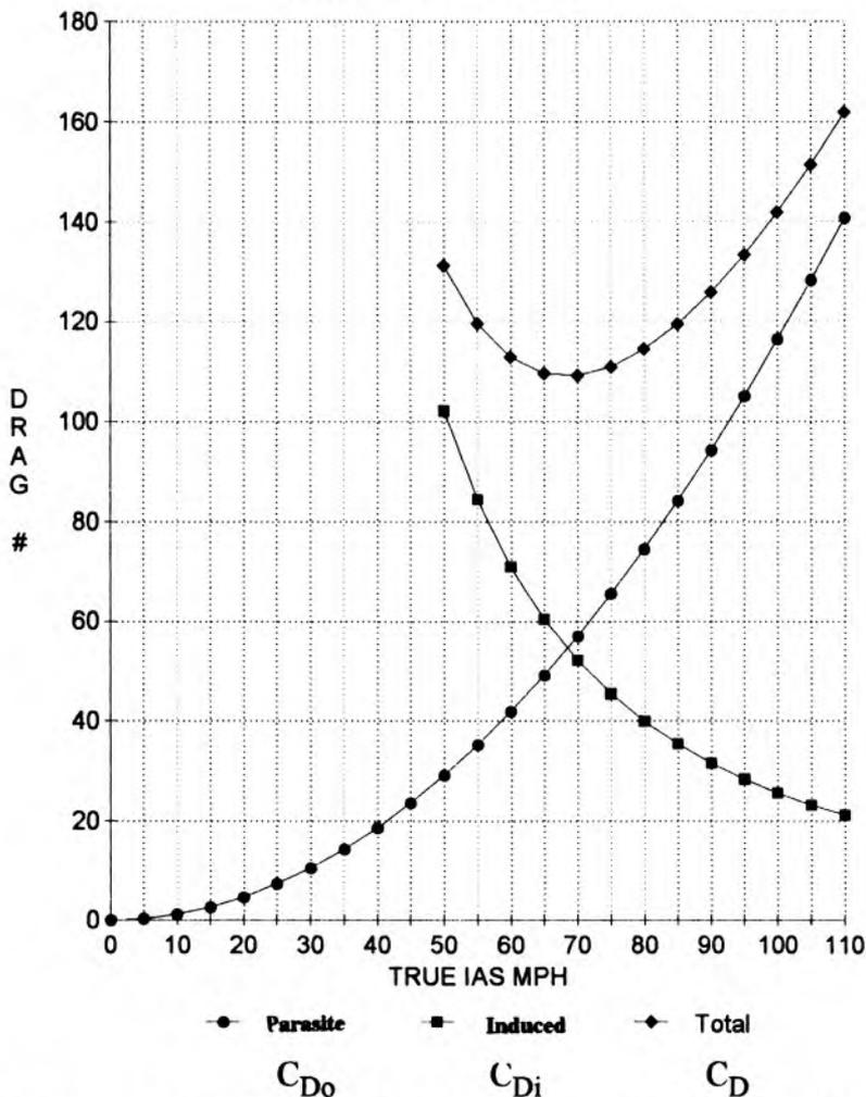
Now, if we just plug that Drag Coefficient into the Basic Drag Formula, (and that means we just multiply it by S q), we get a pretty simple conclusion and expression.--- **INDUCED DRAG equals SPAN LOADING<sup>2</sup> /  $\pi$  e q.** Not only does that give an airplane designer, *and* pilot, an easy way to understand "LIFT DRAG", there is the second great insight. The q<sup>2</sup> in the bottom
