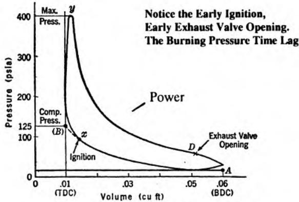
pV Diagram for SI Engine at Wide-Open Throttle.
