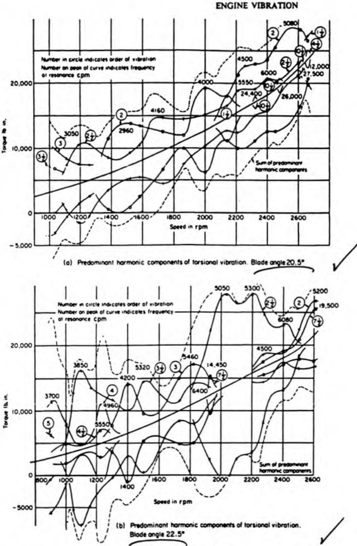
Fig. 8-29. Torque at drive end of crankshaft of Rolls-Royce Merlin II aircraft engine with variable-pitch propeller, 1-to-2 reduction gear (Carter and Forshaw, 8.492).
