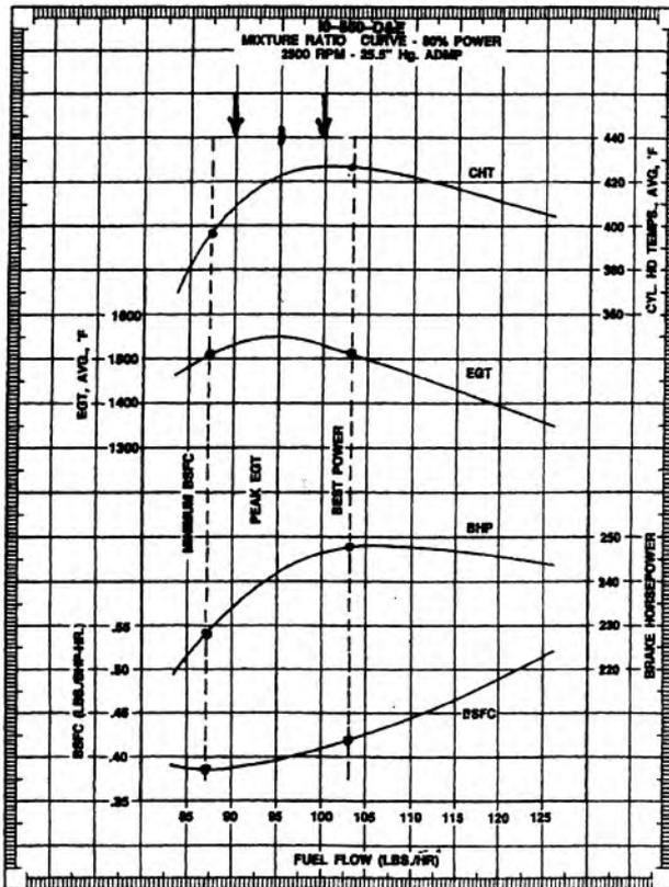
Figure 13-14. Mixture Ratio Curve 80% Power IO-550-D&E
