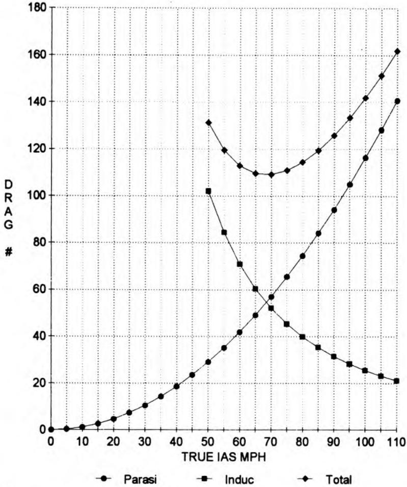
We're going to look at **Minimum Power, Max Endurance, the 2d Optimum** next, but first the thing to start noticing above is how flat the bottom of the drag curve is---but how quick it starts to go vertical! That's where the smart insight is going to come from! At first, as you leave the min. drag IAS, going faster, extra speed is almost free, almost no extra drag! ✓✓ THERE'S AN OPTIMUM POINT to fly, before "drag goes near vertical"!!!! First, let's dispatch that Min. Power Optimum.
