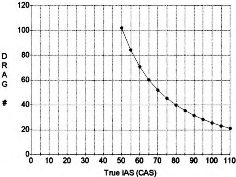
So here's what a  $1/V^2$  curve looks like, as we saw at the end of the last Chapter. It would go to *infinity* at zero MPH, 1, or actually the number that makes the curve plot to the correct values, divided by zero IAS. As speed picks up, it drops like a sinker. To be practical, we just start  $D_i$  at stall speed, to keep it in a realistic range. Recognize though, it never goes to zero!
