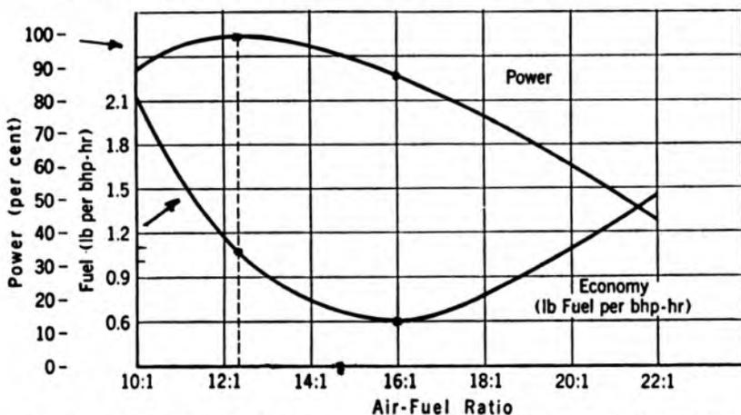
Fig. 123. Variations of Power and Economy of an SI Engine with Carburetor Adjustment (Constant speed and wide-open throttle). ✓
