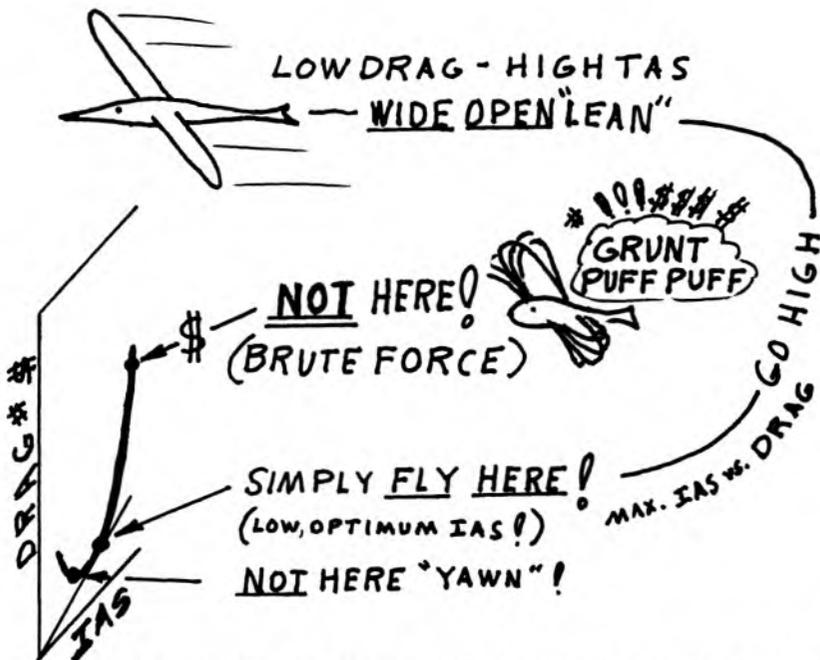
YOU WILL HAVE FOUND THE OPTIMUM L/D, ANGLE OF ATTACK AND "DECK ANGLE", THAT WORKS AT ANY GROSS WEIGHT, ANY ALTITUDE!! YES, THERE IS A "MAGIC ANGLE OF ATTACK", THAT WORKS AT EVERY WEIGHT, EVERY ALTITUDE! IT'S ALL HERE!
