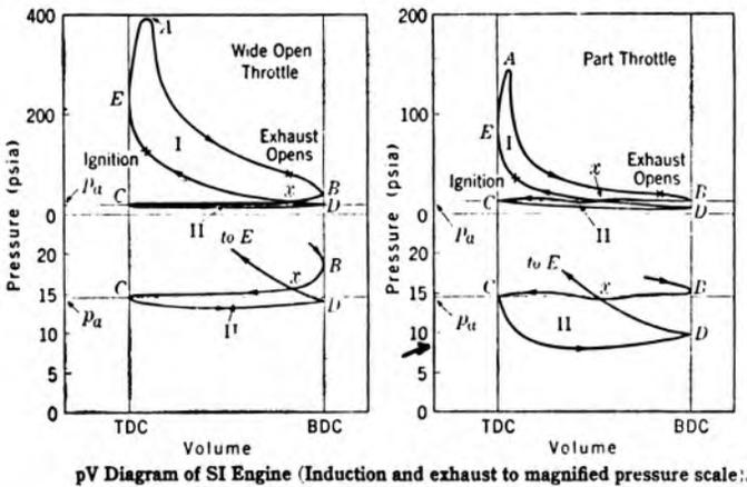
The quite instructive **Throttled PV Diagram**, shows why we don't want to throttle an engine, rather, simply cruise it at Altitude, where less power is available, matching the plane's real cruise need, where we want best efficiency. The Throttled, engine is Required to Pump In it's Working Air --- against the Vacuum created by a throttling plate --- thus work, energy demanded - subtracted from the working Area of the PV Diagram!! It's much better to simply cruise unthrottled at Altitude!
